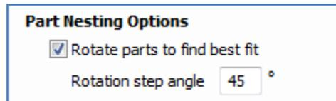
In theory the smaller the specified angle the more options the software will have to fit the shapes together so the more efficient the nesting will be. This does depend on the shape of the vectors though. It should also be noted that the smaller the angle specified the longer the nesting will take to calculate.
