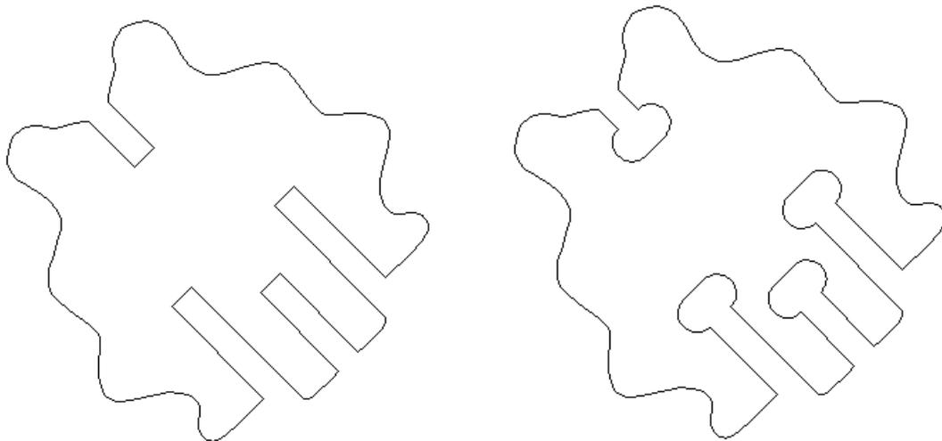
These options are selected within the standard **Create Fillets** menu, the icon for which is located in the **Edit Vectors** area of the **Drawing Menu** as shown in the image below.
