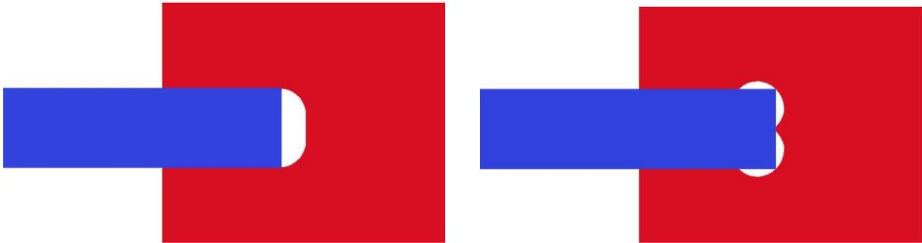
This is a very useful tool for slot-together furniture designs, model aircraft, dinosaurs etc. Below you can see a part from a slot-together dinosaur on the left is the standard part and on the right is the same part with the “T-Bone” style fillets added to these slots. This type of fillet needs to be used when the slot is close in size to the tool diameter.
