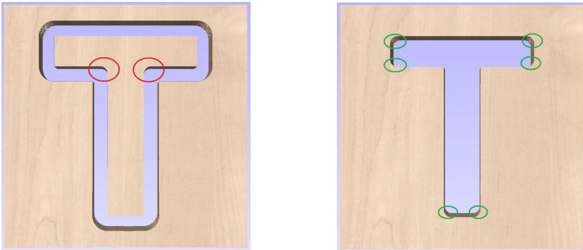
It is not possible to avoid the added radius as it is formed by the tool size and shape. The Inlay function though, will create toolpaths which take the tool radius into account and compensate for it by rounding off the sharp corners so the resulting parts will fit together. This can be seen in the images shown below where the same letter has been cut using the Inlay toolpaths, you can see all corners (internal and external) now have the same radius so they will slot together.
