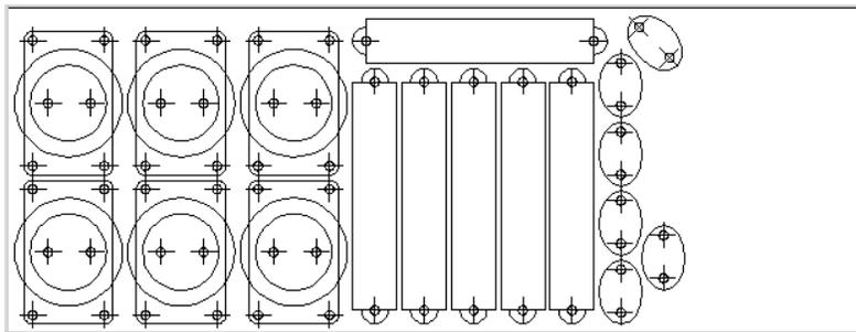
Original vector layers for grouped vectors will be remembered even if the vectors are nested. If nested and then ungrouped the objects within them will go back onto their original layers. This can be useful if you have arrangements of production parts which are on different layers that you need to nest. These might be parts which use layers for different machining operations (drilling, pockets etc.). To nest these you can do the following:
