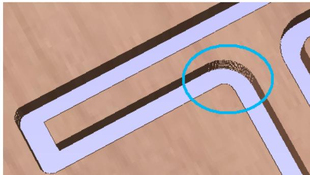
As has been previously discussed it is common to leave an allowance on one or both sides of the inlay, typically when working with letters the allowance would be left on the **Hole** so the size and shape of the lettering itself is not affected any more than necessary.
