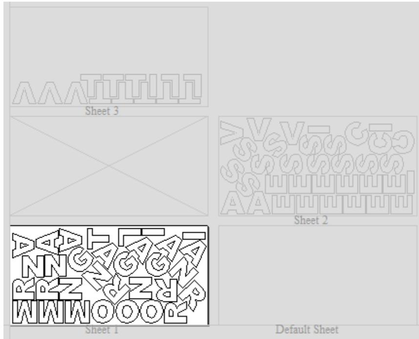
The concept of **Sheets** is very specifically related to machining the finished parts and is not designed to replace layers. **Sheets** should **NOT** be used to organize vectors for modelling or to organize vectors which you intend to use for different machining operations, in those cases the **Layers** should be used to manage the vectors.
