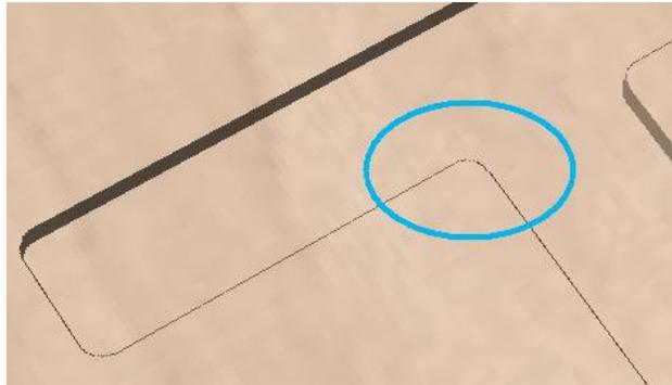
As has been previously discussed it is common to leave an allowance on one or both sides of the inlay, typically when working with letters the allowance would be left on the **Pocket** so the size and shape of the lettering itself is not affected any more than necessary.
