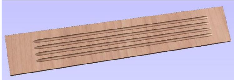
Another good application for straight flutes is the markings on a draining board (for Solid Surface fabricators) or on a cutting block (for carving meat) such as the one shown below, sloping down to allow liquid to be directed.
