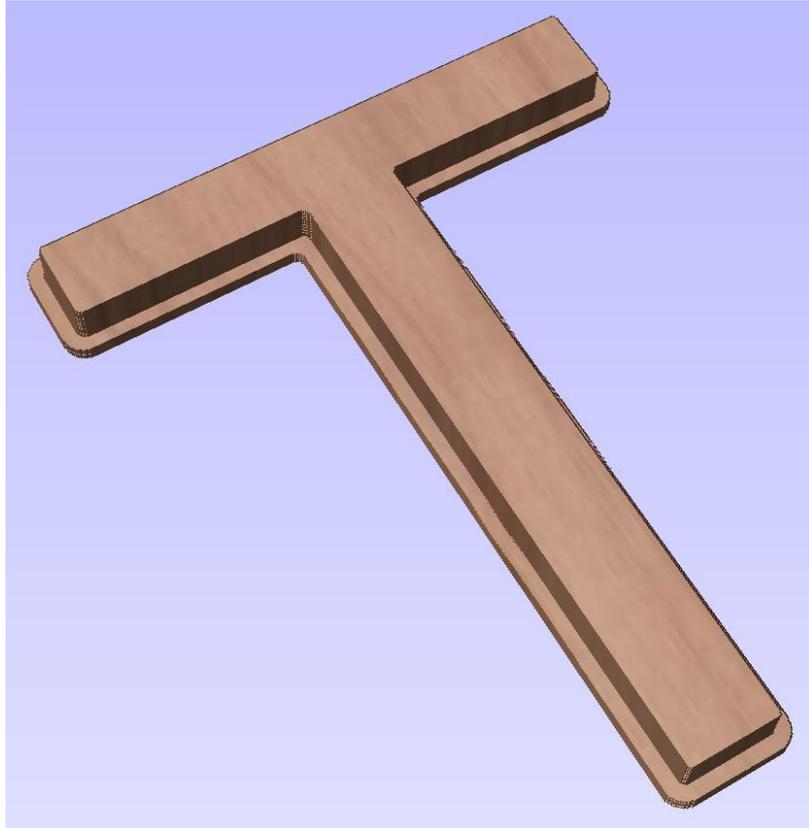
The image shown above shows a Stepped Male Inlay created in 1 inch thick material with a **0.75” Step Depth** and a **0.3” Step Width**.
