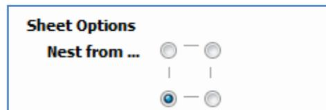
Each node corresponds to the respective corner of the Material or the selected boundary vector. The first nested parts will be placed in that corner and the shapes fitted according to the **Nest Direction** specified (see section below).
