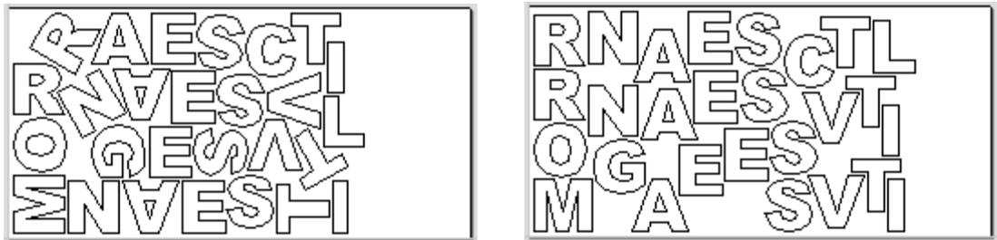
The image above and left shows the letters nested with 30 degree rotation and the image above right shows the same letters nested with NO rotation. As you can see by allowing the rotation the software can fit the letters into a smaller area. In this case it is not a huge difference but the more shapes there are and depending on the style of the shapes it could be a bigger margin.
