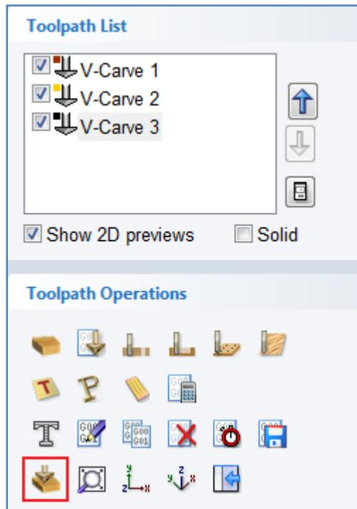
When this icon is clicked (or immediately after a toolpath is calculated) then the **Preview** menu will be shown. The new options for defining the fill color are contained in the **Machined Area Color** area of the form highlighted with a red box in the image below.
